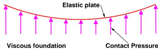
Figure 19:4: Elastic plate resting on Viscous foundation
