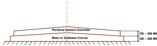
Figure 19:3: Typical Cross section of Rigid pavement
