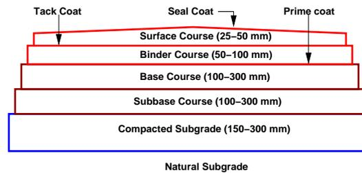
Figure 19:2: Typical cross section of a flexible pavement
