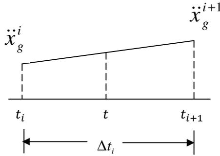
Figure 3.6: Time step for Runge-Kutta method
