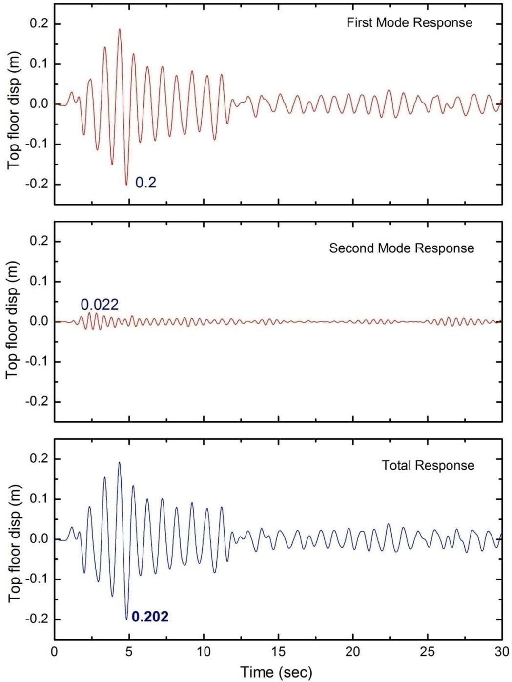
Figure 3.13 Top floor displacement response of two DOF system of Example 3.6.
