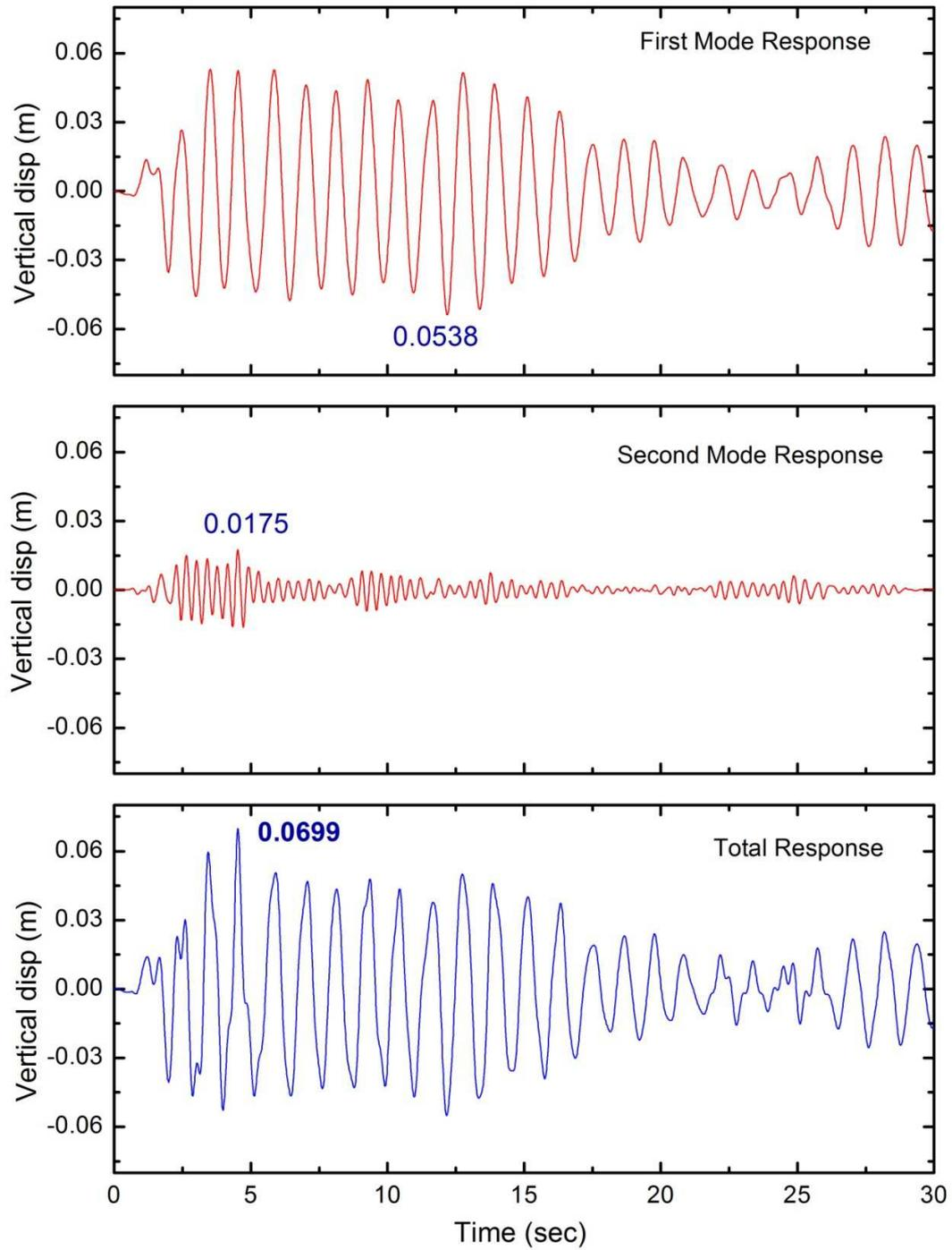
Figure 3.17 Vertical displacement response of the Industrial Structure of Example 3.7.
