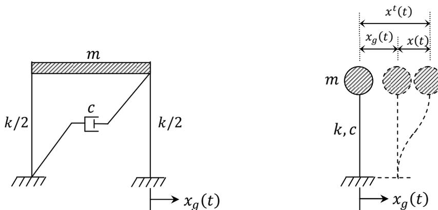
Figure 5.1 (a) SDOF system (b) Lumped mass model of SDOF
