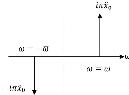
Figure 3.8 Graphical Representation of  $\text{FT}[-\ddot{x}_o \sin \bar{\omega}t]$ .
