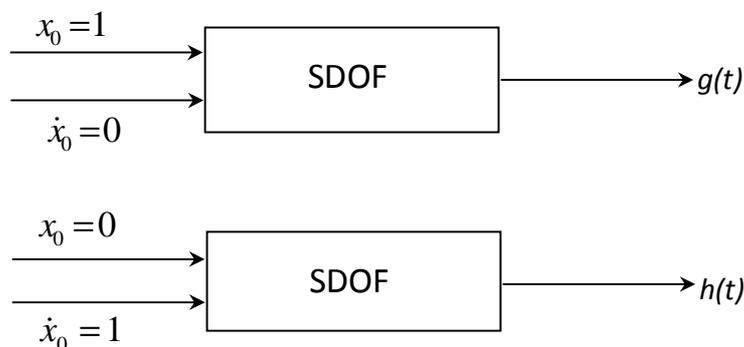
Figure 3.2 Response of SDOF system to initial unit displacement and velocity.
