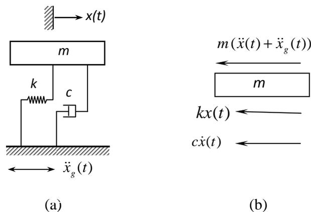
Figure 3.1 (a) SDOF system (b) Free body diagram.
