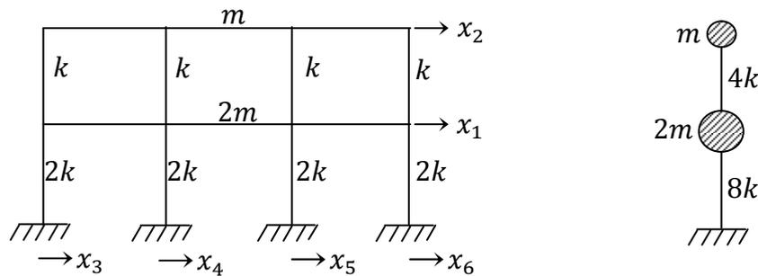
Figure 5.5 (a) A multi-bay portal frame (b) Lumped mass model of frame
