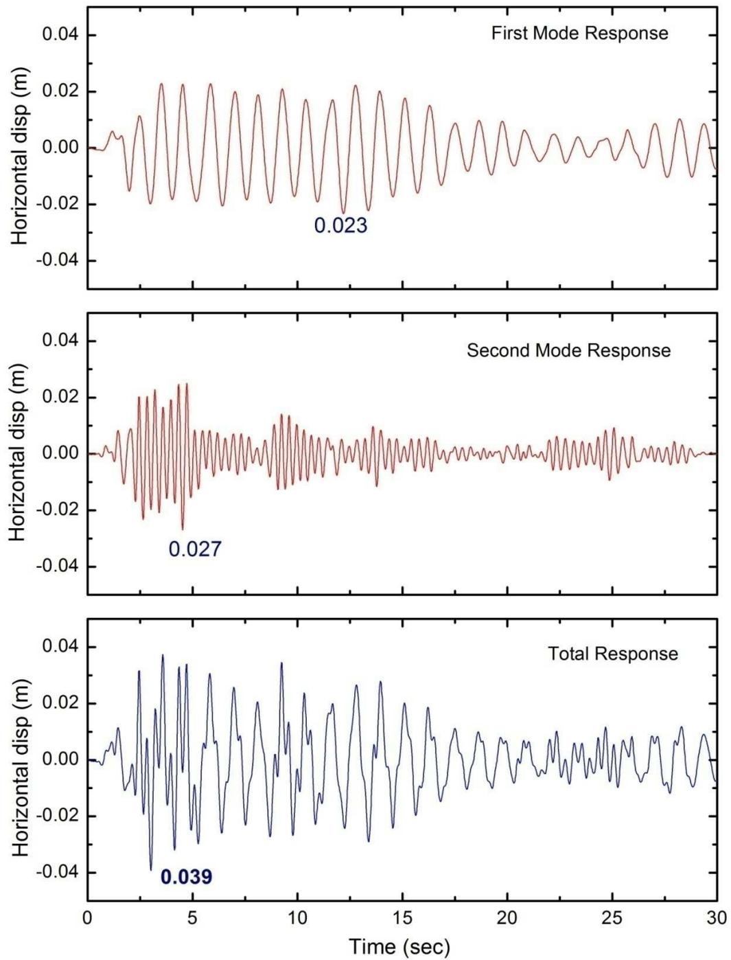
Figure 3.16 Horizontal displacement response of the Industrial Structure of Example 3.7.
