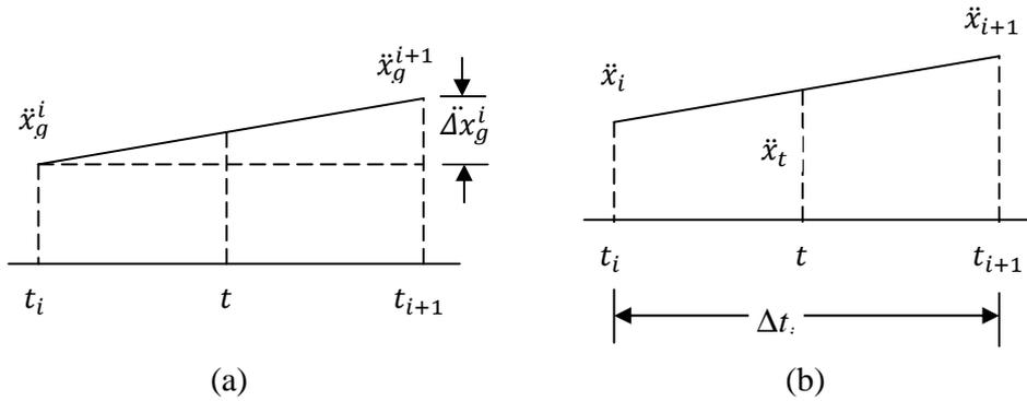
Figure 3.5 (a) Linear ground acceleration, (b) Linear relative acceleration of SDOF system over time step,  $\Delta t_i$ .
