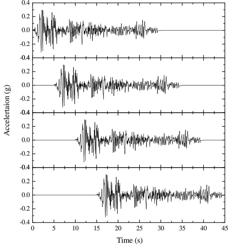
Figures 5.12 Acceleration time history of El-Centro, 1940 earthquake for four supports with time delay of 5 s between supports
