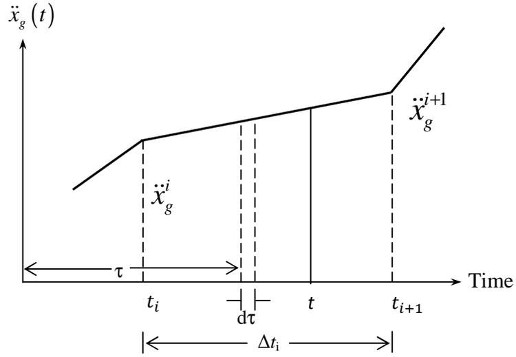
Figure 3.4 Linear variation of ground acceleration across chosen time step  $\Delta t_i$  .
