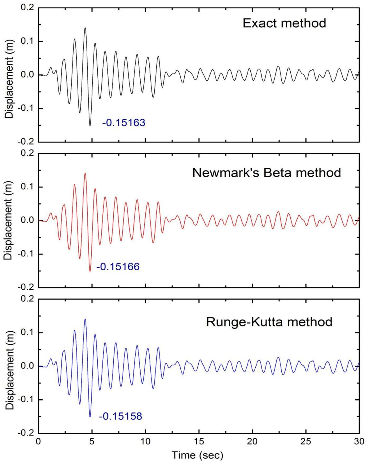
Figure 3.10 Response of SDOF system of Example 3.5 by various methods.
