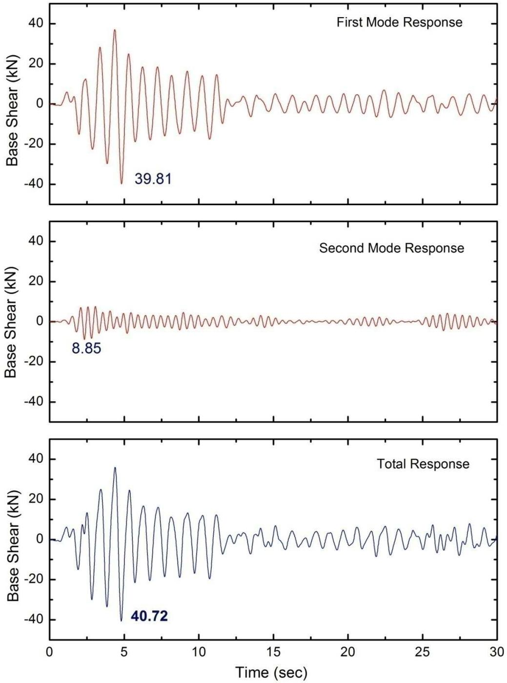
Figure 3.14 Base shear response of two DOF system of Example 3.6.
