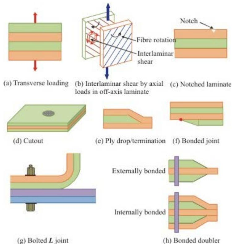
**Figure 6.5: Situations conducive for delamination**
