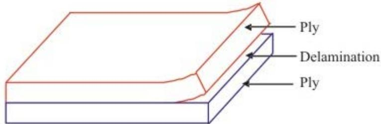
**Figure 6.4: Macro-level damage mechanism (Delamination)**
