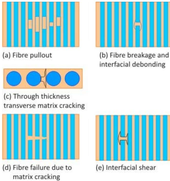
**Figure 6.3: Fibre-matrix coupled failure mechanisms**
