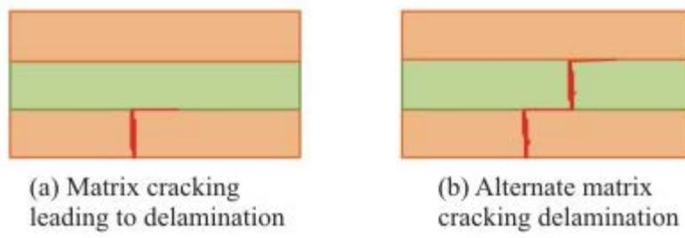
**Figure 6.6: Coupled micro-macro damage mechanisms**
