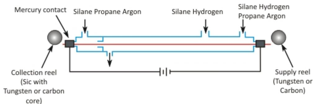
**Figure 1.9: Schematic of reactors for silicon carbide fibres by Chemical Vapour Deposition**
