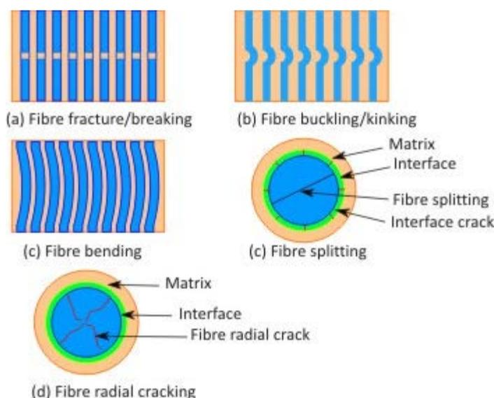
**Figure 6.1: Fibre-level damage mechanisms**
