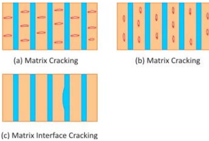
**Figure 6.2: Matrix-level damage mechanisms**
