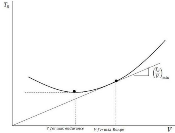
Figure 1: Thrust required curve to determine  $[T_R/V]_{min}$
