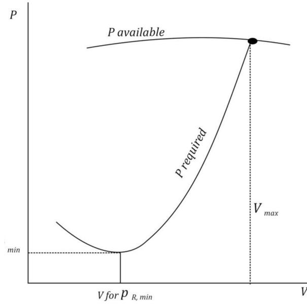
Figure 1: Power available and power required as a function of speed
