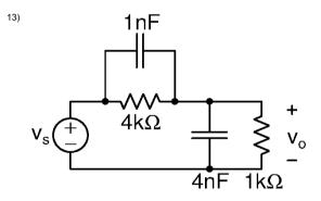
In the circuit above,  $v_s(t) = \cos(10^6 t)$  V. The forced response is  $V_p \cos(10^6 t + \phi)$ . Determine  $V_p$  and  $\phi$ .
