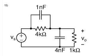
In the circuit above,  $v_s(t) = \cos(10^5 t)$  V. The forced response is  $V_p \cos(10^5 t + \phi)$ . Determine  $V_p$  and  $\phi$ .
