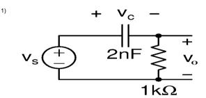
In the circuit above,  $v_c(0^-) = 1 \text{ V}$ .  $v_s(t) = 2 \exp(-t/1 \,\mu\text{s}) \text{ V}$ . The output for t > 0 is of the following form:
