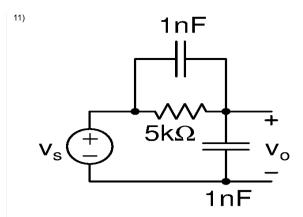
In the circuit above,  $v_s(t) = \sin(10^5 t)$  V. The forced response is  $V_p \cos(10^5 t + \phi)$ . Determine  $V_p$  and  $\phi$ .
