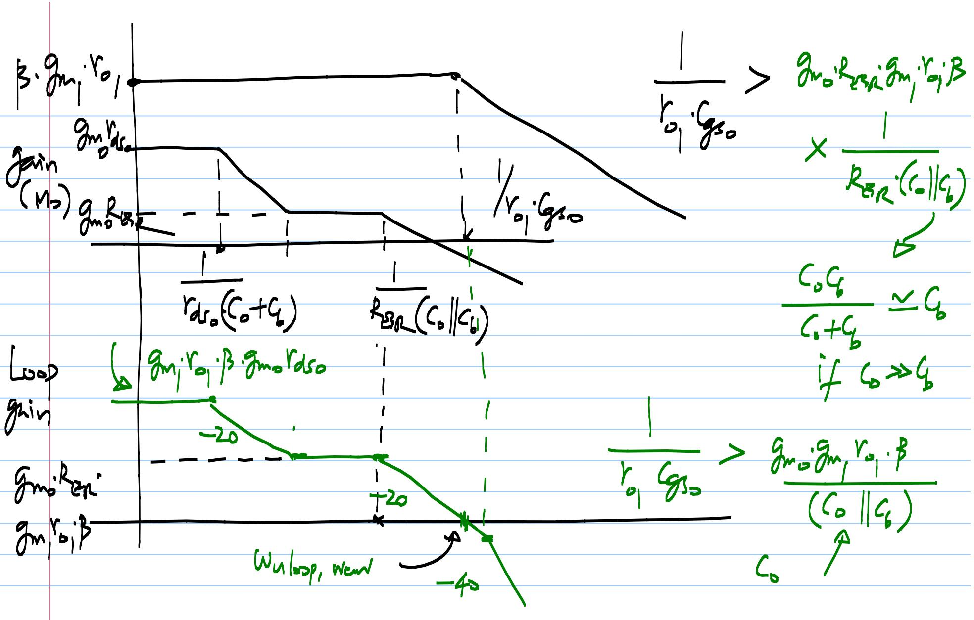
$$r_{o_1} < \sqrt{\frac{C_o || C_b}{C_{gs_0}} \cdot g_m, g_{m_0} \cdot \beta}$$
