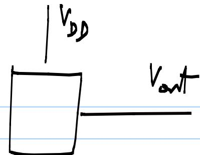
\*  $\frac{\Delta V_{out}}{\Delta I_L} = R_{out}$  must be small (load regulation)
