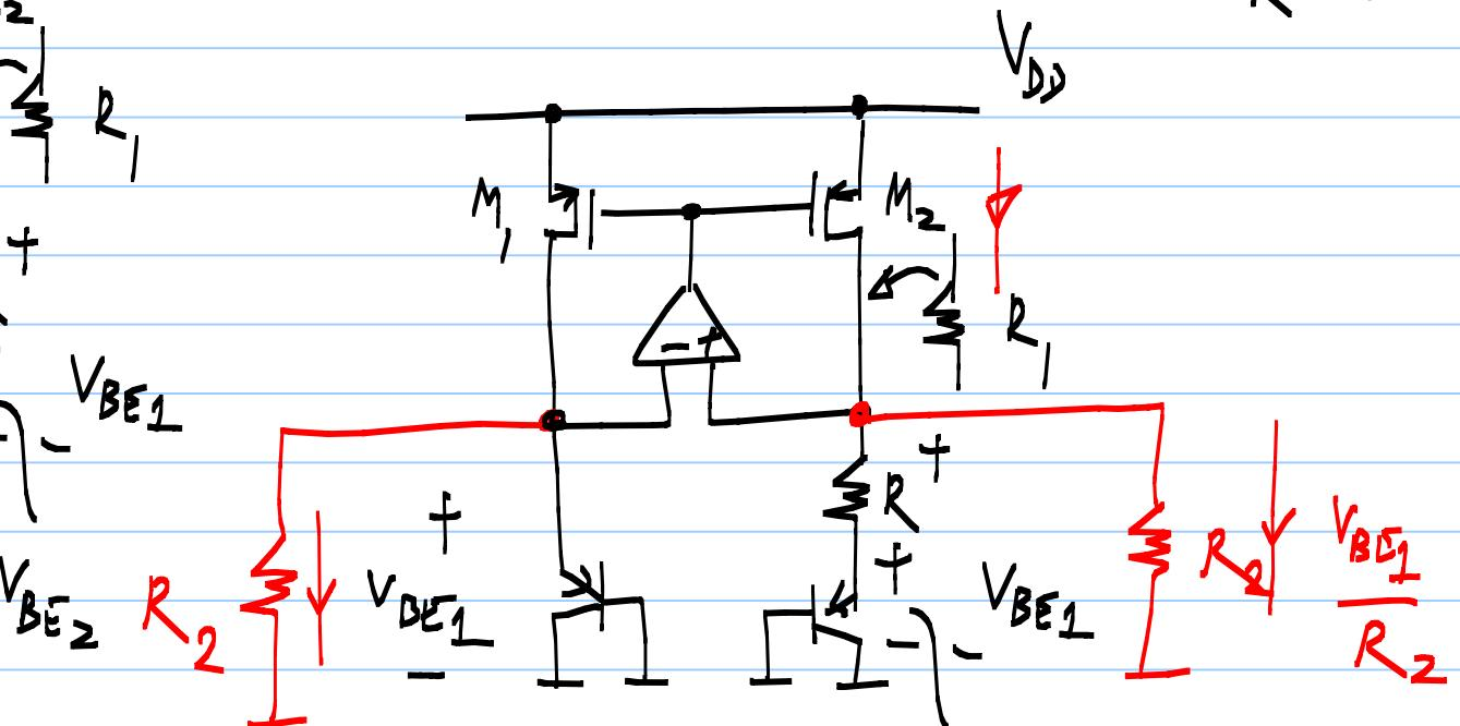
Currents in  $M_{1,2}$ :  $\frac{V_T \ln(N)}{R} + \frac{V_{BE1}}{R_2} = \frac{V_{BE2} \left[ V_{BE1} + V_T \ln(N) \frac{R_2}{R} \right]}{R_2}$
