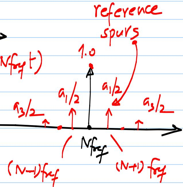
$$\frac{a_1}{2} = 10^{-2} \quad \left[ \text{reference spur} = 40\text{dB below the component at } Nf_{ref} \right]$$
