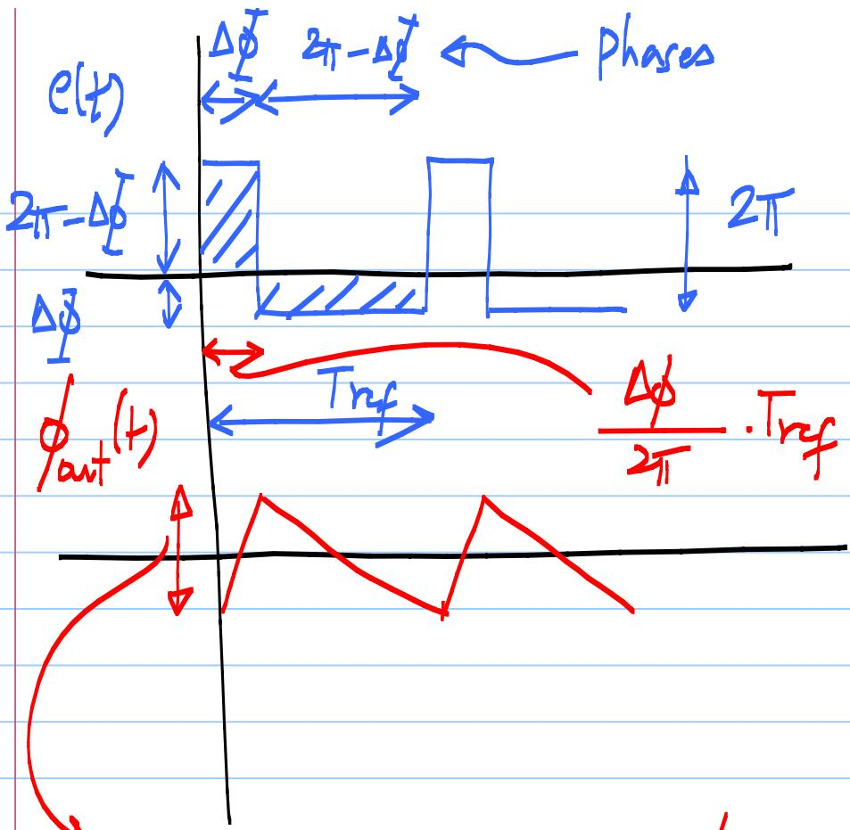
$$2\pi K_{VCO} K_{PD} = (2\pi - \Delta\phi) \cdot \frac{\Delta\phi}{2\pi} \cdot T_{ref}$$
