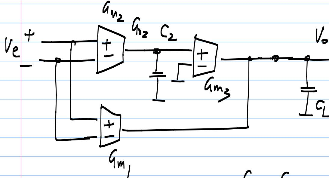
$$\frac{V_o}{V_e} = \frac{G_{m1} + \frac{G_{m2} \cdot G_{m3}}{sC_2}}{sC_L} = \frac{G_{m1}}{sC_L} \left( 1 + \frac{G_{m2} G_{m3}}{G_{m1} sC_2} \right)$$
