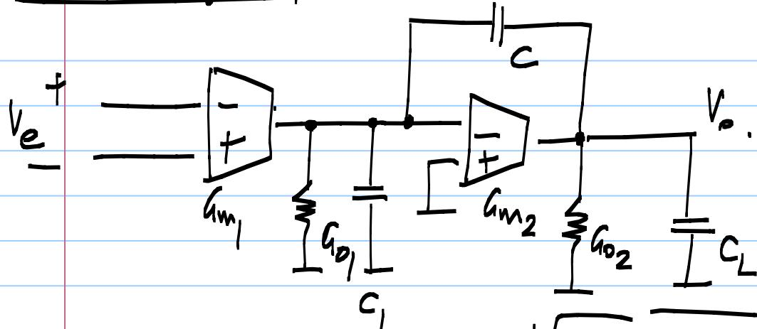
$$A_o = g_{m_1} g_{m_2} / R_{o_1} R_{o_2}$$
