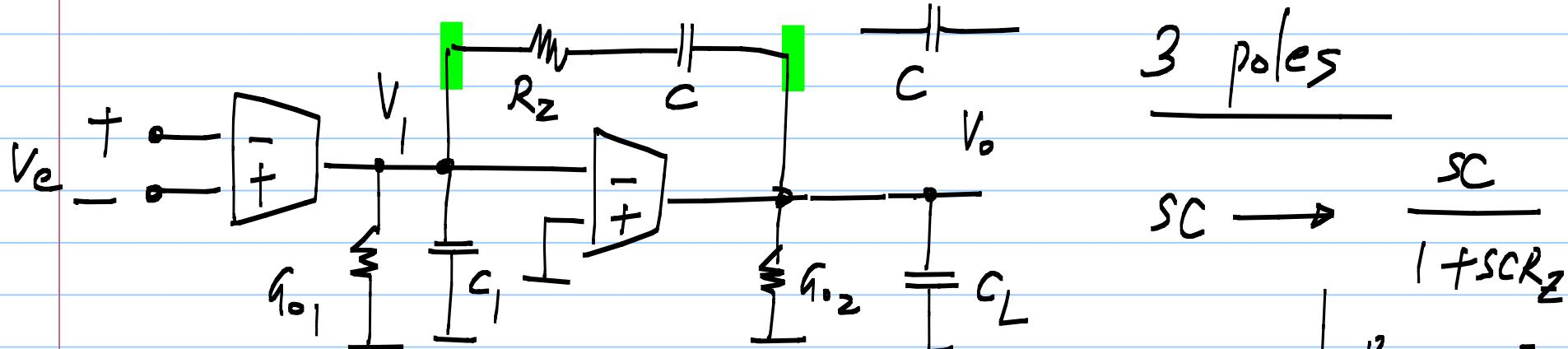
$$\begin{bmatrix} SC_1 + \frac{SC}{1 + SCR_Z} + g_{o_1} \\ g_{m_2} - \frac{SC}{1 + SCR_Z} \end{bmatrix} = \begin{bmatrix} V_1 \\ V_o \end{bmatrix} = \begin{bmatrix} -g_m V_e \\ 0 \end{bmatrix} \quad \left| \begin{array}{l} R_z \quad z_1 \\ = \frac{1}{g_{m_2}} \quad \infty \\ < \frac{1}{g_{m_2}} \quad R_{HP} \\ > \frac{1}{g_{m_2}} \quad l_{HP} \end{array} \right.$$
