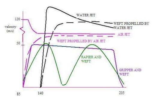
Angular Position of crank in degrees
