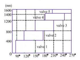
Ans Number of jets controlled by each of the valves 1, 2 and 3 is four, whereas each of the two valves 4 and 5 control two jets. Thus there are in all 16 jets. The loom runs at 600 rpm completing one cycle of operation in 0.1 seconds. Each of the five valves operate over 60° of crank shaft rotation which takes (1/60) s. In other words each of the 16 jets blows for (1/60) s accounting for a cumulative blowing time of (4/15) s. Thus air consumption per loom cycle amounts to (400/15) = 26.66 cc.
