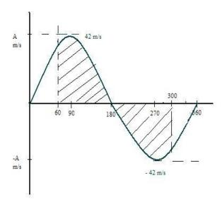
Both Dewas and Gabler rapier inserting a single pick would exhibit the same velocity profile.
