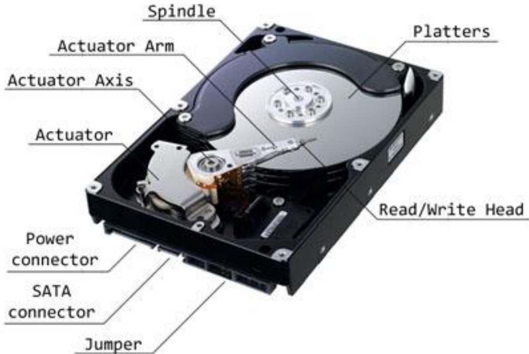
Figure 28.1: Photographic view of the hard disk drive [1].
