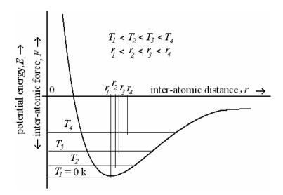
• If a very deep energy trough caused by strong atomic bonding is characteristic of the material, the atoms separate to a lesser and the material has low linear coefficient of thermal expansion. This relationship also suggests that materials having a high melting temperature – also due to strong atomic bonds – have low thermal expansion coefficients.
