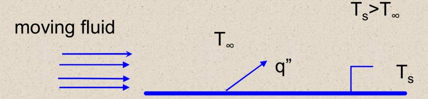
Energy transferred by diffusion + bulk motion of fluid
