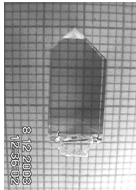
Figure 5.13. The size and the quality of the crystal grown in platform geometry during free convection experiment.
