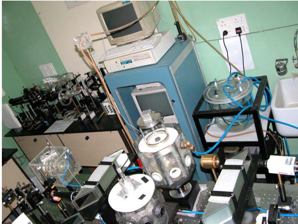
Figure 3.9. Full view of the experimental set up involving the interferometer, growth cells, thermostated water recirculation system and camera.
