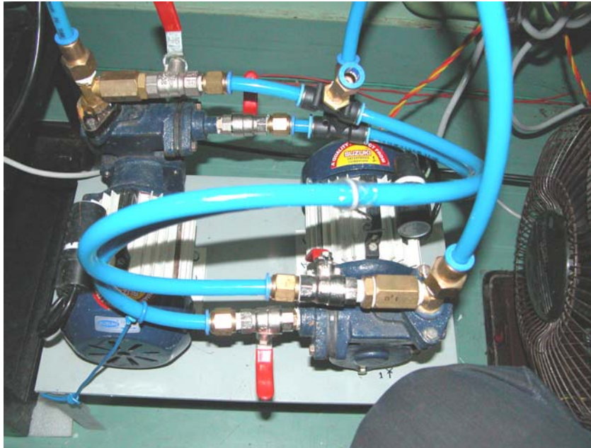
Figure 3.7. Pump-and-valve system for recirculating thermostated water through the cell.
