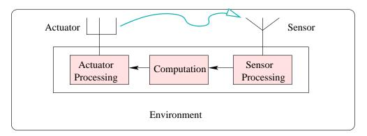
Figure 9: Feedback Structure of Real-Time Systems
