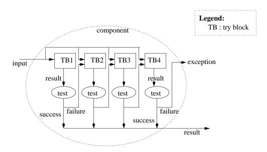
Figure 12: A Software Fault-Tolerance Scheme Using Recovery Blocks
