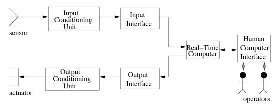
Figure 3: A Model of a Real-Time System
