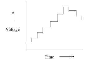
Figure 6: Analog Voltage Converted to Discrete Form
