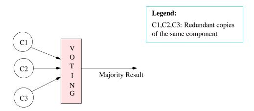
Figure 11: Schematic Representation of TMR
