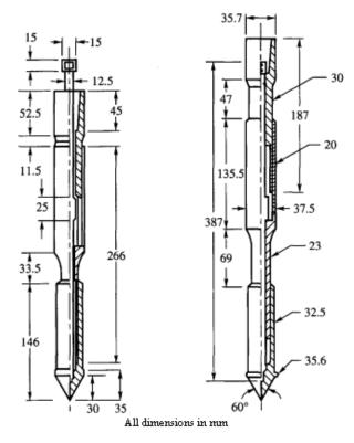
Fig 1.6: Standard cone Penetrometer
