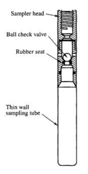
Fig. 1.5: Shelby tube sampler
