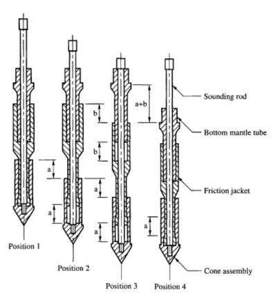
Fig 1.7: Operation of cone Penetrometer
