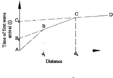
Slope of AB =  $\frac{1}{V_1}$
