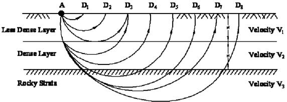
(a) Schematic Representation of seismic refraction method
