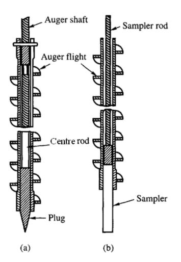
Figure 1.2 Hollow-stem auger (a) Plugged while advancing the auger, and (b) plug removed and sampler inserted to sample soil below auger
