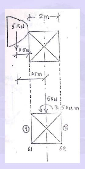
The moment will cause compression on the windward side and tension on the leeward side.
