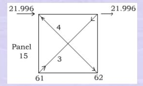
The lateral force of 43.992 kn is shared by the diagonal bracings equally and the tension diagonal is considered as effective taking moment about joint 62
