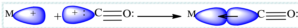
Figure: Formation of a M \leftarrow CO \sigma -bond in metal carbonyls.
