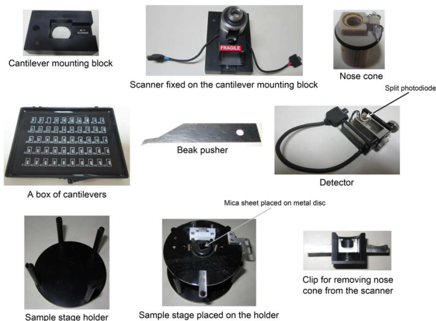
Figure 36.5 Components and accessories of an atomic force microscope from Agilent Technologies
