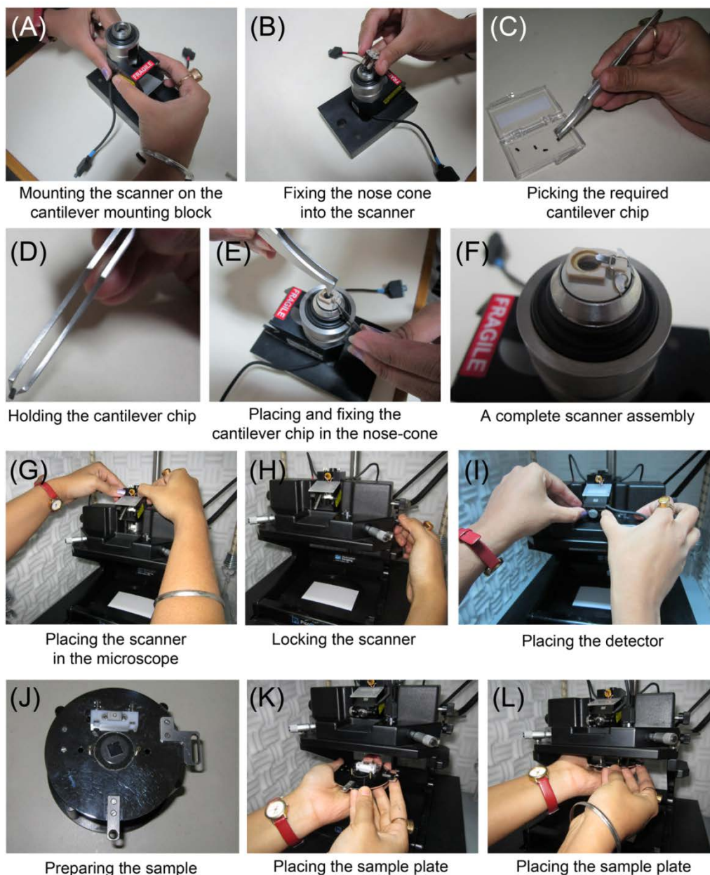
Figure 36.6 Steps showing fixing the different components of the AFM. The steps are discussed in the text
